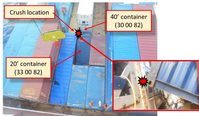
Ref: Top view of accident site and location where ASD was crushed. TSIB report - MIB/MAI/CAS.046
