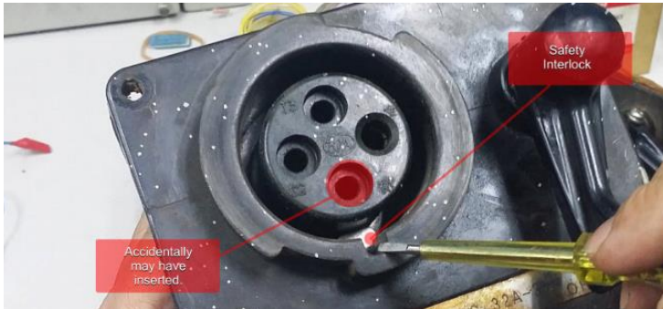
Ref: Faulty socket and mechanism MPA SRS e-Bulletin 2015/ISSUE 03
