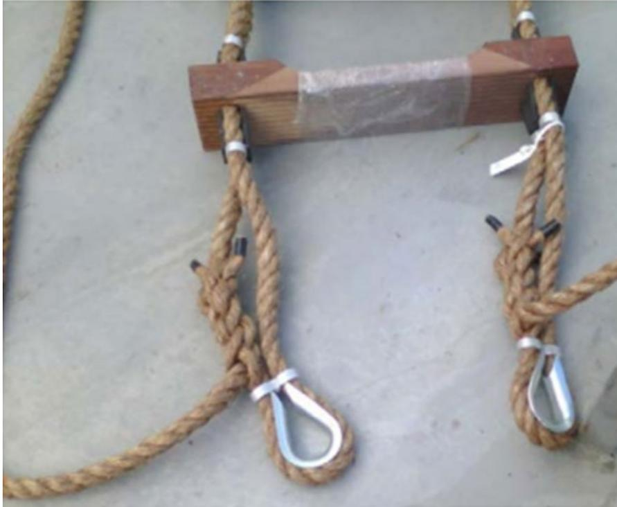
Pilot ladders constructed like this are considered non-compliant by AMSA. Vessel operators and vessel masters are recommended to check their pilot ladders for splices in side ropes.
