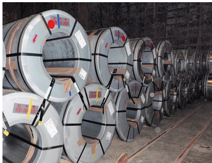
Typical loading and securing method of steel coils
