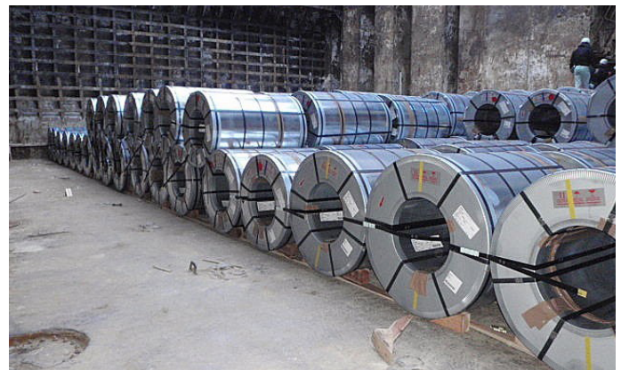
Stowage of steel coils
