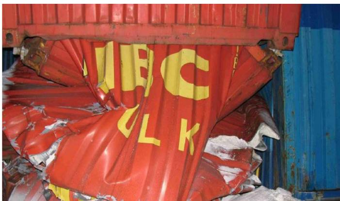
Crushed container at the bottom of the stack, Ref: [MAIB Report No 21/2007](#)
