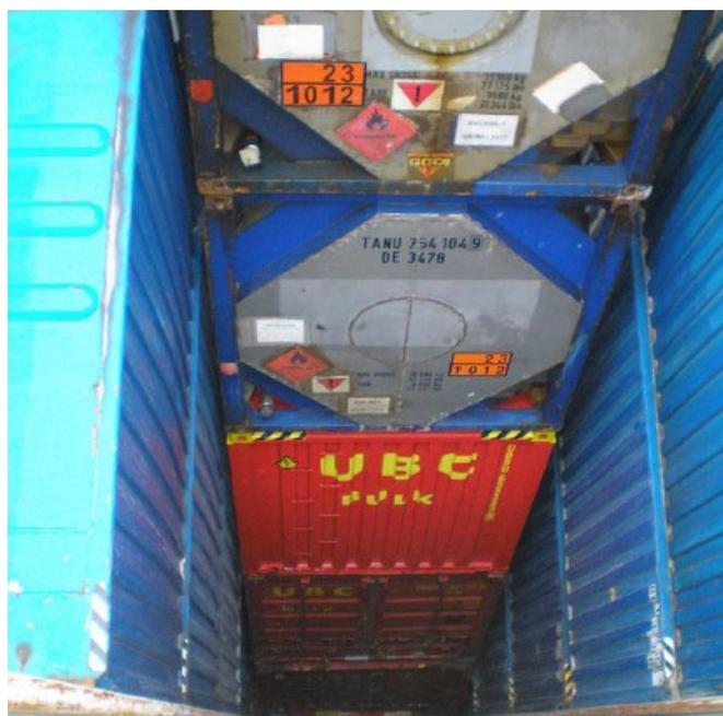
Looking down on the aft end of the collapsed stack of containers, Ref: [MAIB Report No 21/2007](#)
