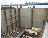
destructive testing (NDT). Any welds that fail NDT are to be ground out and rewelded prior to re-testing by NDT. Where cell guide structures and supporting brackets are to be used as lashing points, it must be verified that these are suitable to withstand the dynamic loads expected in the lashings.
