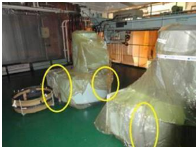
Lashed spare auxiliary blowers in the engine-room TMSI Report: 18/2019
