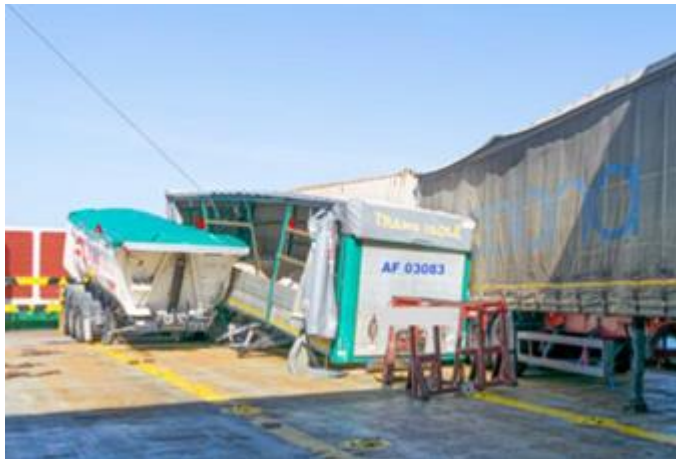
Damage to trailers behind deckhouse- (Ref: TMSI Report: 17/2020)
