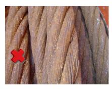
If the wire rope is worn such that the diameter has decreased then it should be discarded. Again various standards specify different limits on allowable loss of rope diameter, stating that the rope should be discarded if between 6 and 10% of the original diameter of the rope has been lost.
