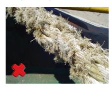
Areas of actinic degradation should also be inspected closely to assess the rope's integrity.
