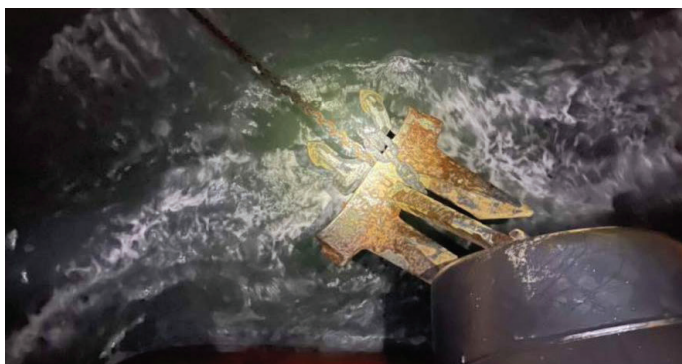
Anchor fouled with abandoned anchor and chain
