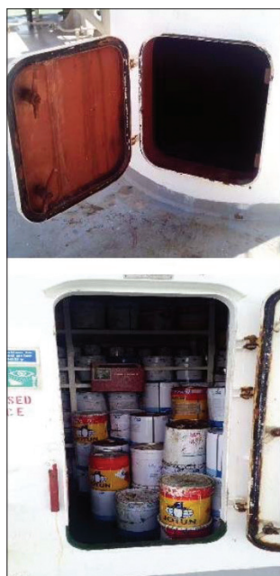
Paint stored in crane pedestal
