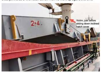
to the aft panel No.2-3 (indicated by an arrow in the photograph), and started cleaning at the starboard side of panel No.2-3. While moving toward the port side, out of sight of the crewmember tending the hose, he slid down the incline, through the gap in the hatches, and fell at least 17 metres to the hold tank top. A cry was heard and the crewmember tending the hose began searching, only to see his colleague lying on the tank top of the hold in the middle of the hatch area.
