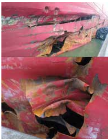
Collision damage with rock barge
