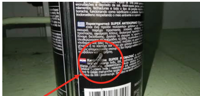
Hole where welding spark initiated a flame burst
