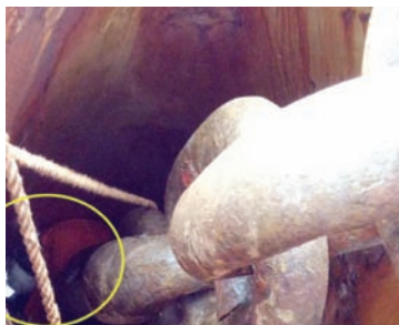
Top: stuck fluke Bottom: Crew member pinned in hawsepipe
