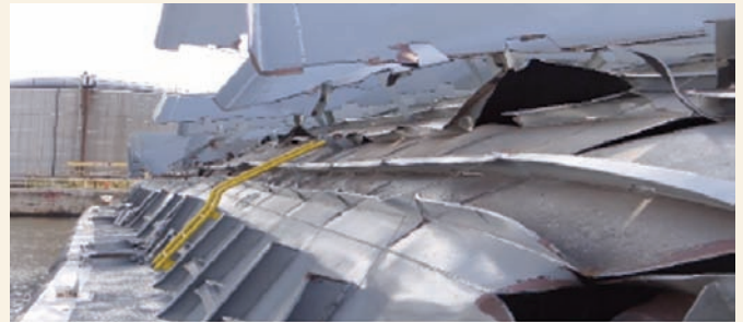
Breached cargo tank
