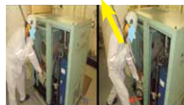
Motor gets stuck Motor comes free
