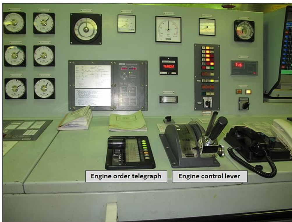
Anna Smile ECR engine order telegraph and main engine control lever.
