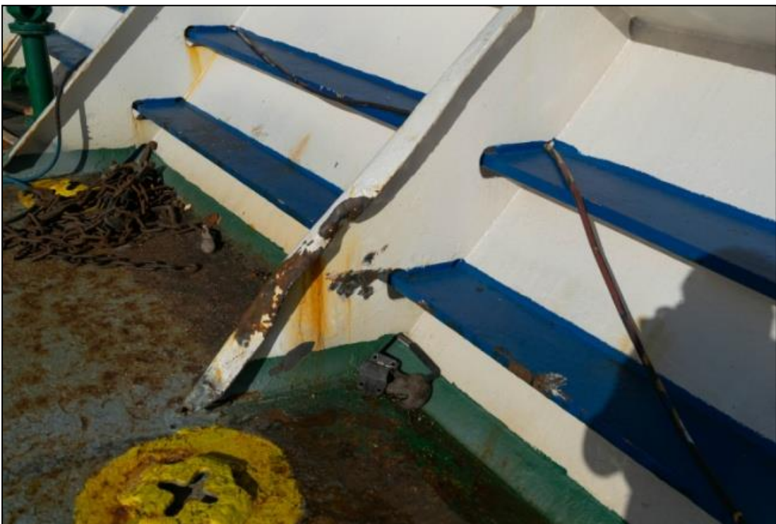
Figure 22: Damaged bulwark stiffener
