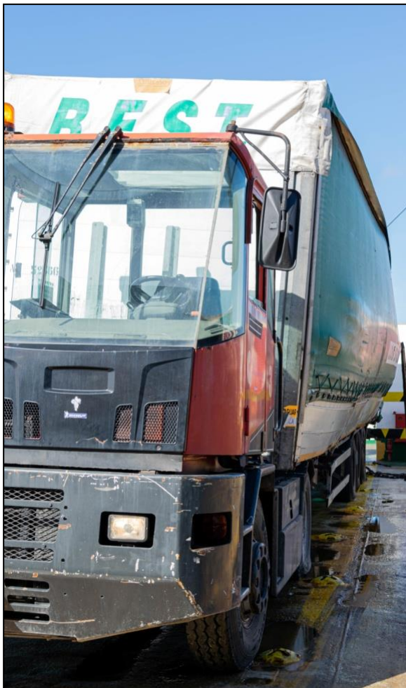
Figures 26a and 26b: Bulging of the sides due to internal cargo shift
