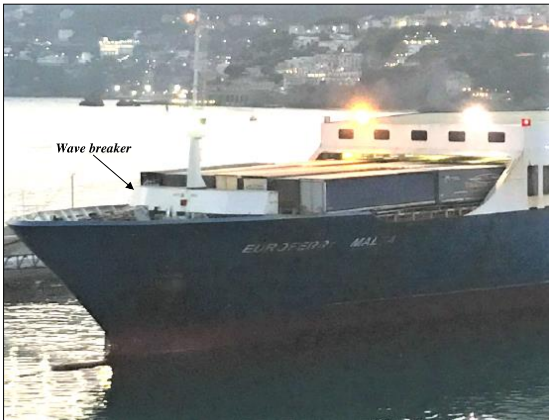
Figure 5: Deckhouse serving as a wave breaker
