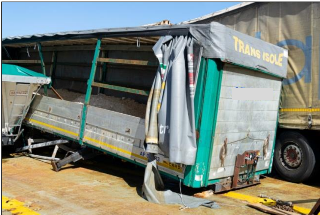
Figure 17: Damaged landing gear of trailer B
