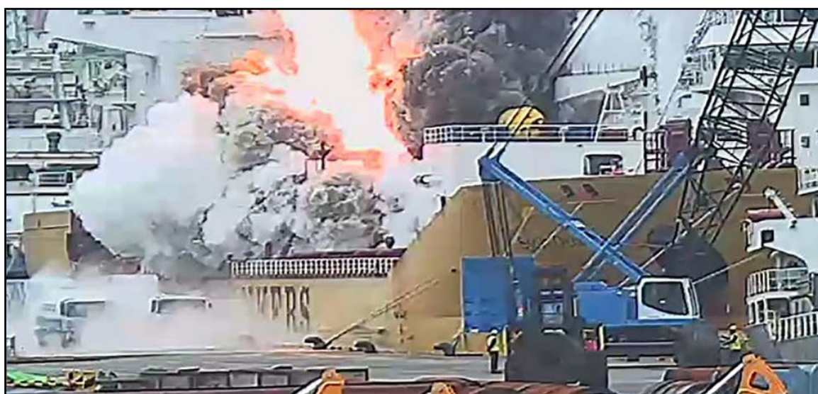
Figure 5: CCTV still showing vapour ignition
