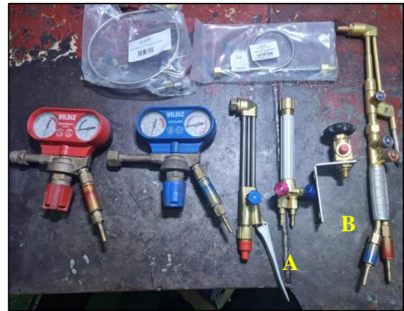
Figure 9: Spare pressure regulators fitted with flashback arrestors, a torch fitted with non-return valves (A) and a torch fitted with non-return valves with flashback arrestors (B)
