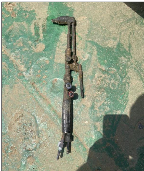
Figure 4: The damaged torch
