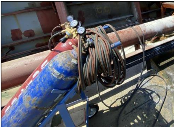
Figure 6: The oxy-acetylene set used for the task
