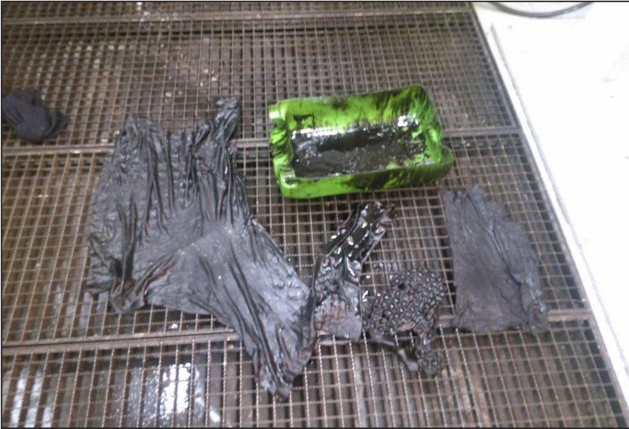
Figure 1: Rags found in the drain tank
