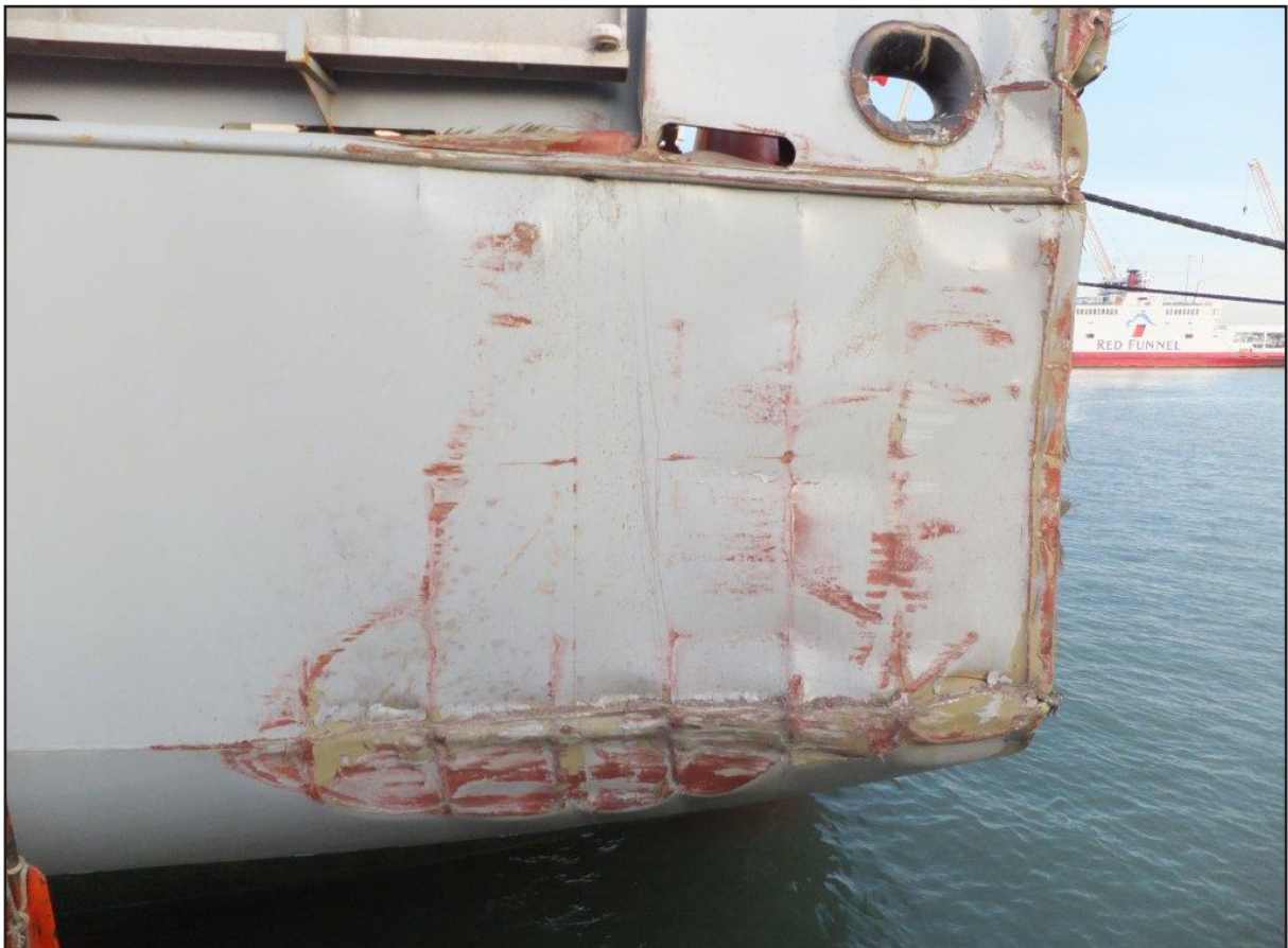
Damage sustained to the general cargo vessel
