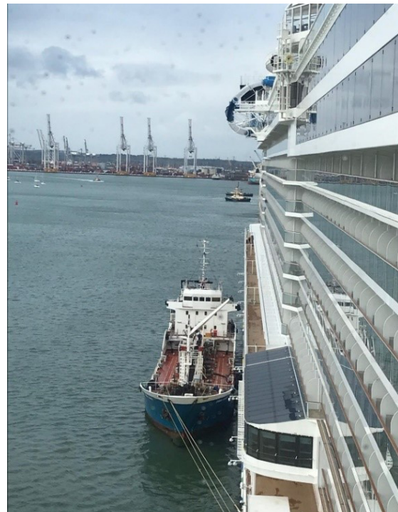
Bunker in progress
