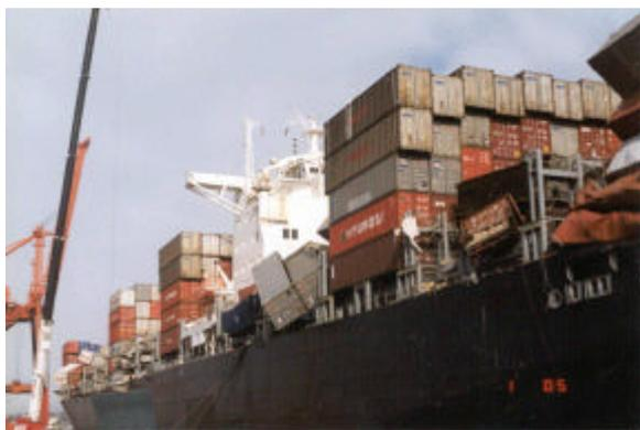
**Figure 1 Representative Container Damage**
