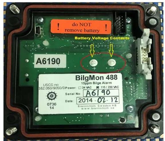
failure combined with a low back-up battery voltage, the unit is locked down and the display reads "RTC check: FAILED." [Click here for the applicable manual.](#)
