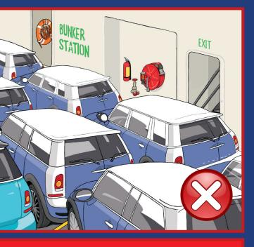
Do not obstruct safe accessways and emergency exits on RO-RO spaces and/or vehicle decks
