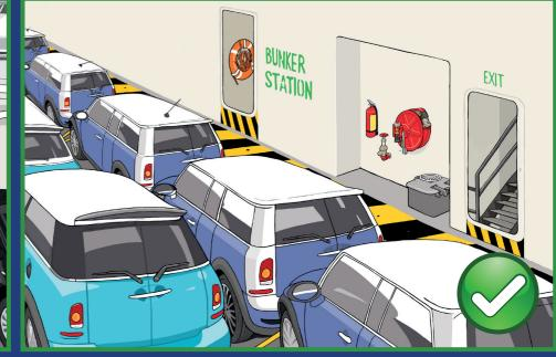
In accordance with SOLAS Regulations, all firefighting and emergency equipment shall be maintained in good working order and be readily available and accessible for immediate use. Escape routes, stairways, emergency exits and safe exits around and on Ro-Ro Spaces and/or vehicle decks must be kept clear at all times.
