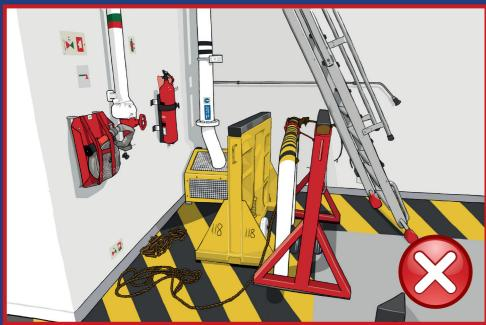
Do not obstruct emergency equipment on RO-RO spaces and/or vehicle decks
