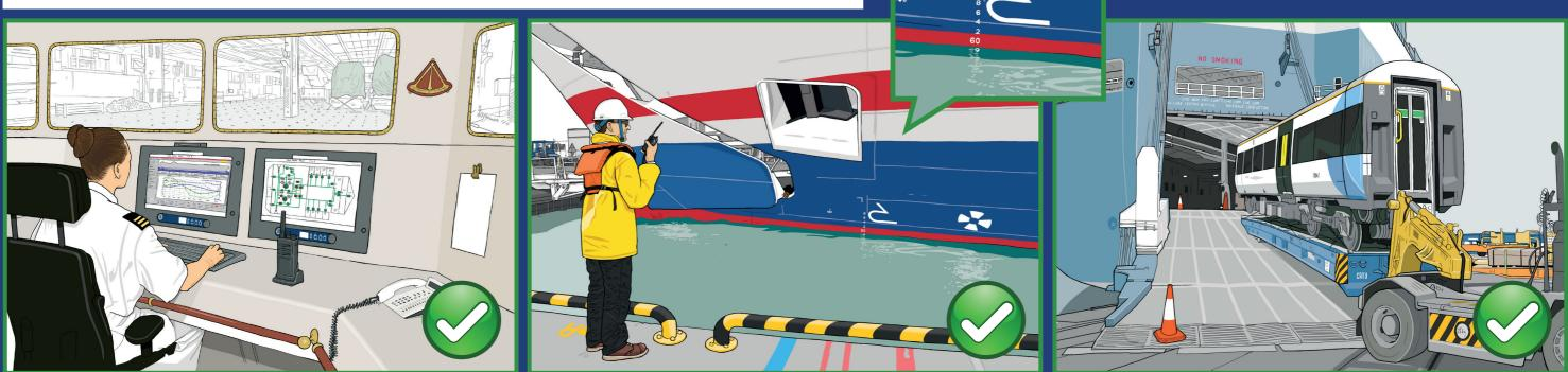
Continuously monitor ship draught and stability, particularly when loading large, high and heavy cargo. DO NOT Depart until intact stability has been checked and verified for entire voyage. ALL ballast operations to be in accordance with regulatory requirements.
