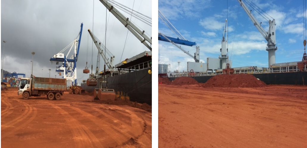
Figure 5: Loading with vessel's cranes and grabs
