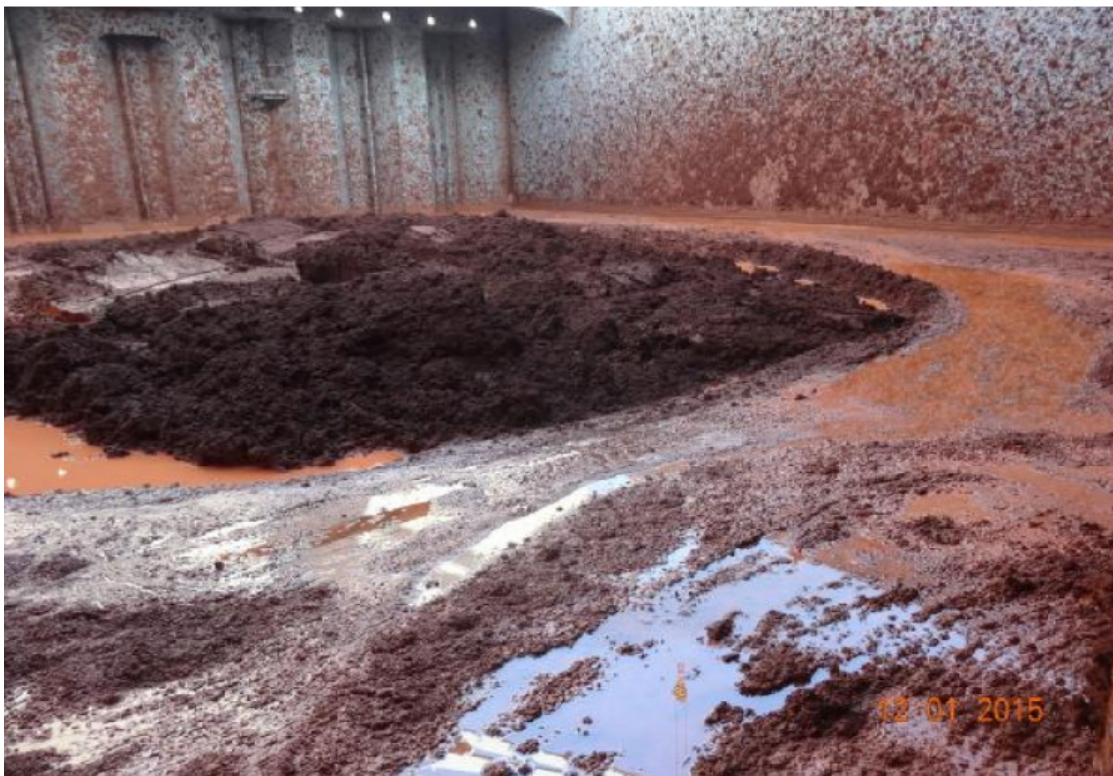
Figure 34: General view across hold No. 4 on board 'm.v Orchid Island', note extensive splatter on bulk head
