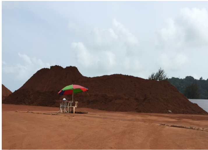
Figure 10: Uncovered stockpile in port
