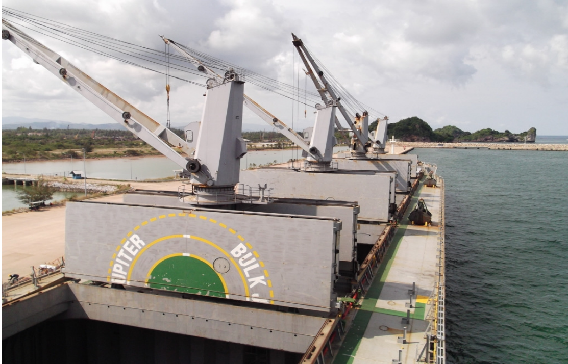
Figure 30: Bulk Jupiter cargo hatches and grab cranes (photo date 25/02/2012)
