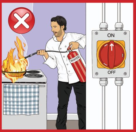
First switch off power, always use an appropriate extinguisher or fire blanket subject to fire types.
