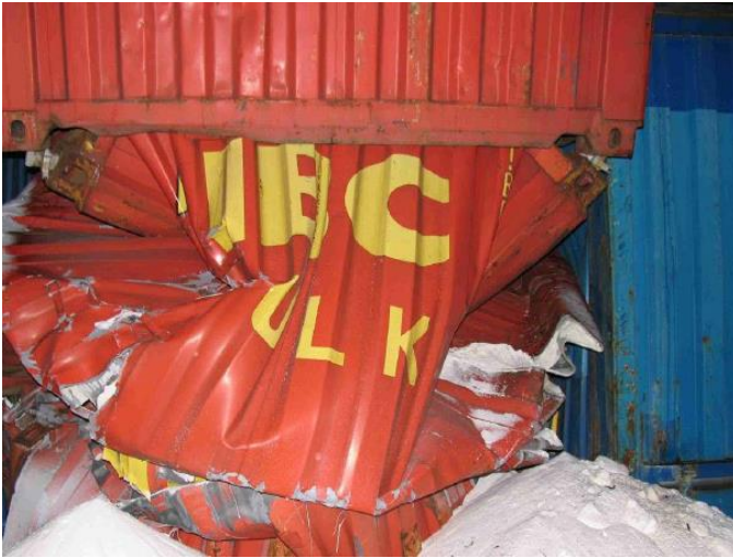
Crushed container at the bottom of the stack. Ref: MAIB Report No 21/2007
