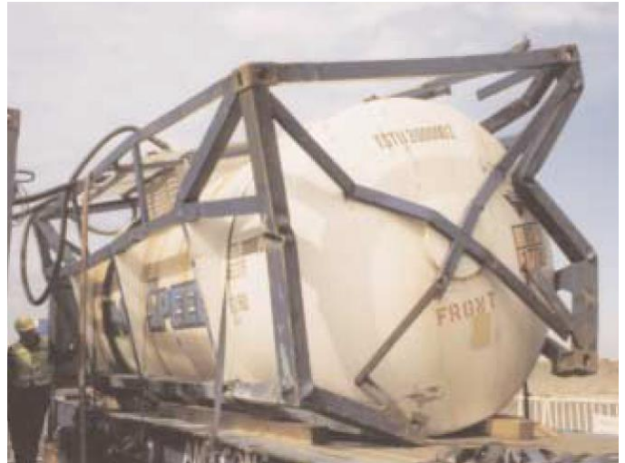
Damaged front end frame - Ref: MAIB report no 37/2002
