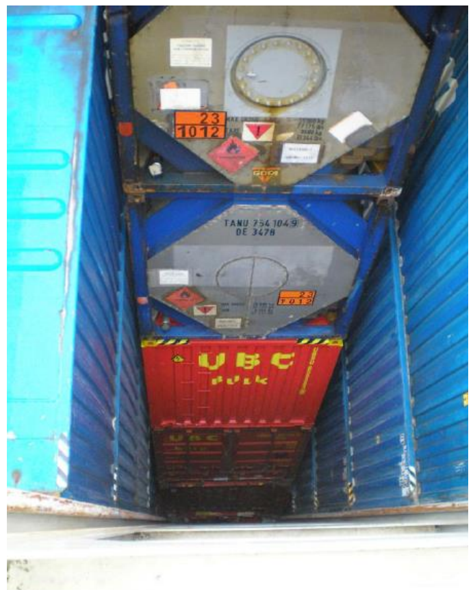
Looking down on the aft end of the collapsed stack of containers, Ref: MAIB Report No 21/2007
