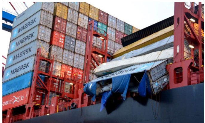
Container with polystyrene balls hanging overside Bay 26: Ref: Joint investigation report - MSC Zoe 01 - 02 Jan 2019
