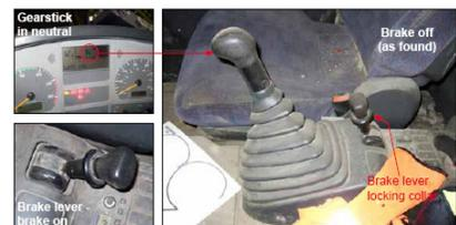
2. The tractor and trailer unit had not been parked or secured in accordance with the requirements of the vessel's own Cargo Securing Manual or in line with the guidance contained in the IMO Code of Safe Practice for Cargo Stowage and Securing (CSS Code).
