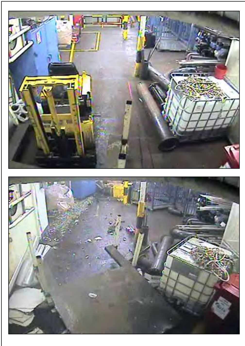
Deck 3 handling area and crew main access, before and after the large rolls
