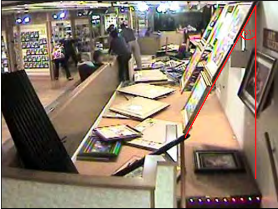
Art Gallery and Photo Gallery, Deck 9, at the largest recorded roll angle
