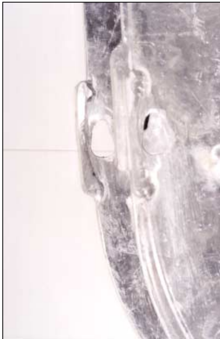
Photograph of ruptured sockets
