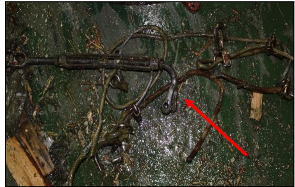
Figure 9: Damaged lashings of auxiliary blowers. Bent turnbuckle shown by the red arrow. (Photo courtesy of the USCG)
