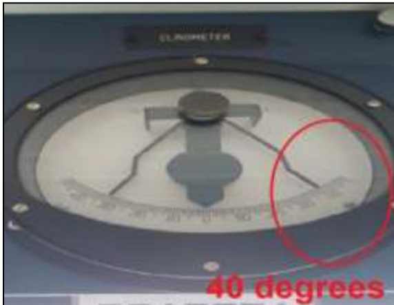
Figure 11: Clinometer on the bridge indicating a roll of almost 40°
