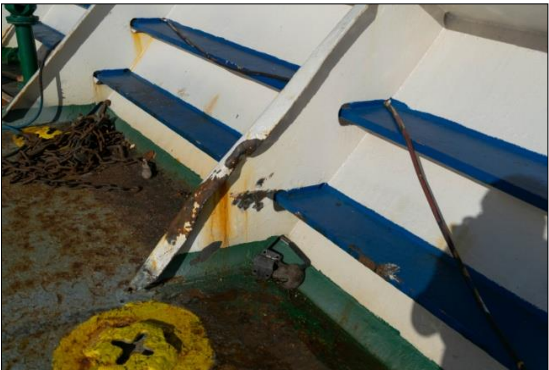
Figure 22: Damaged bulwark stiffener
