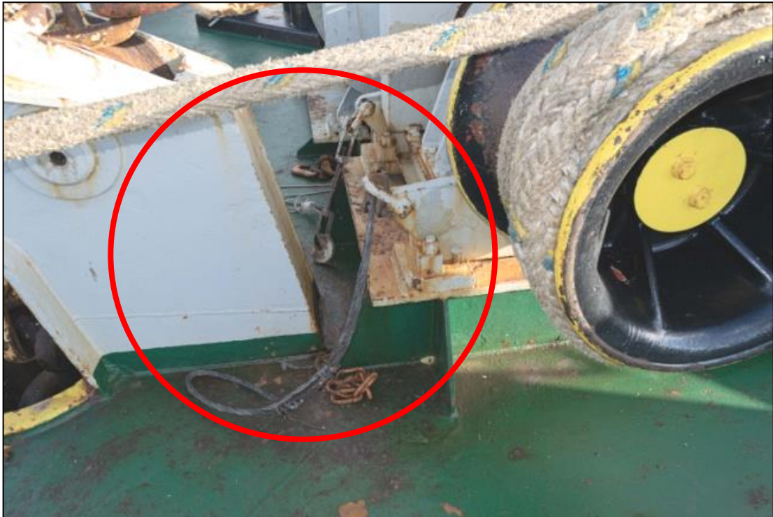
Figure 8: Additional securing arrangement
