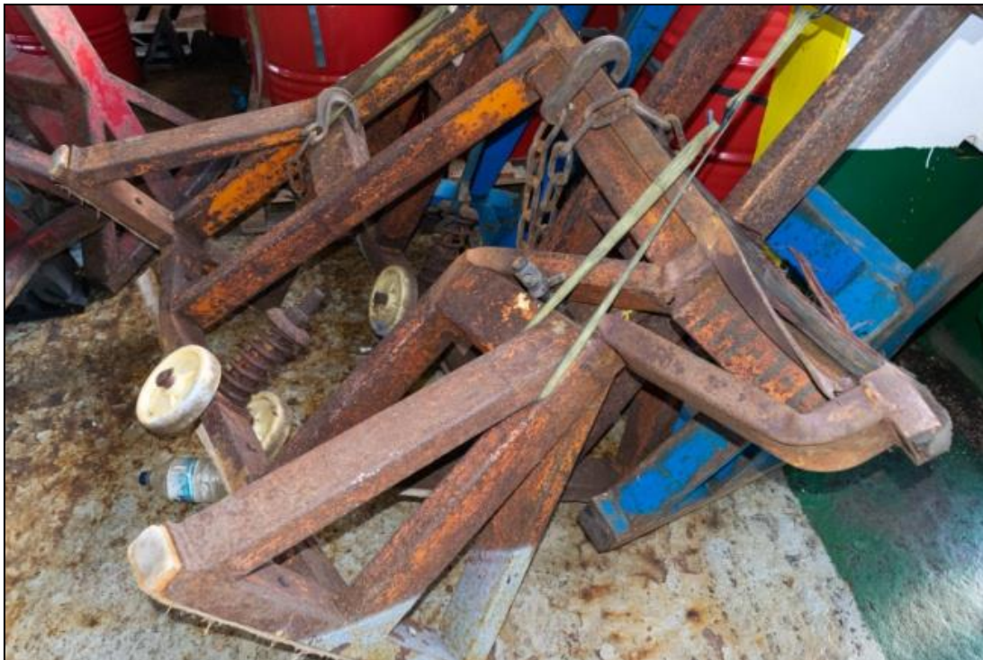
Figure 20: A damaged trestle
