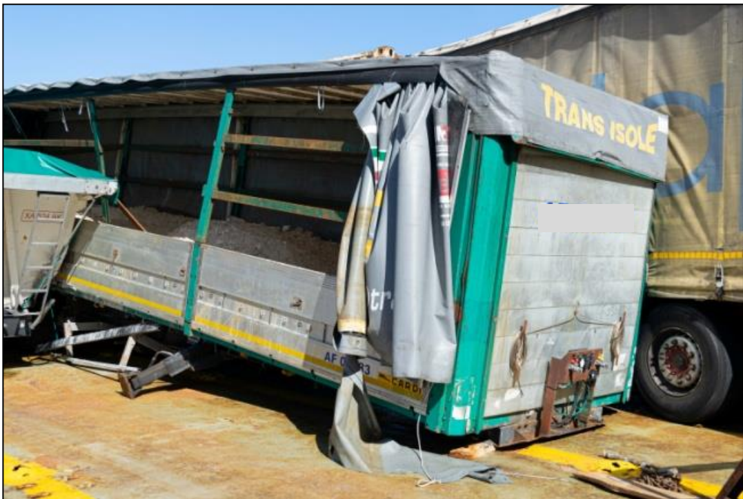
Figure 17: Damaged landing gear of trailer B
