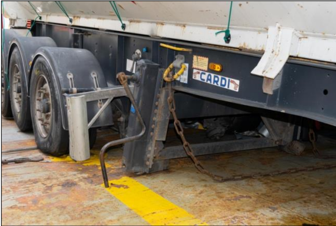
Figure 16: Damaged landing gear of trailer A
