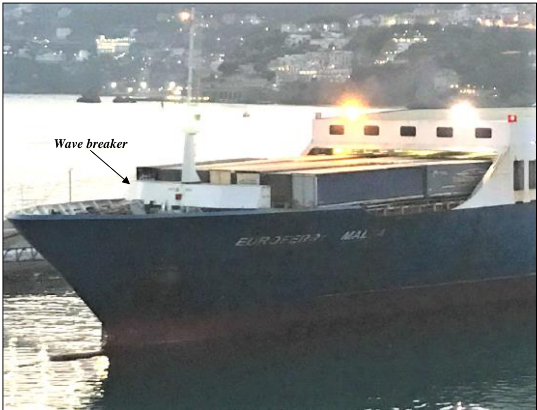
Figure 5: Deckhouse serving as a wave breaker
