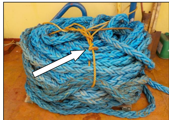
Figure 3: One of the mooring ropes on the poop deck, secured on a pallet and an adjacent fitting
